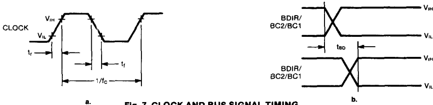
Fig. 7 CLOCK AND BUS SIGNAL TIMING
