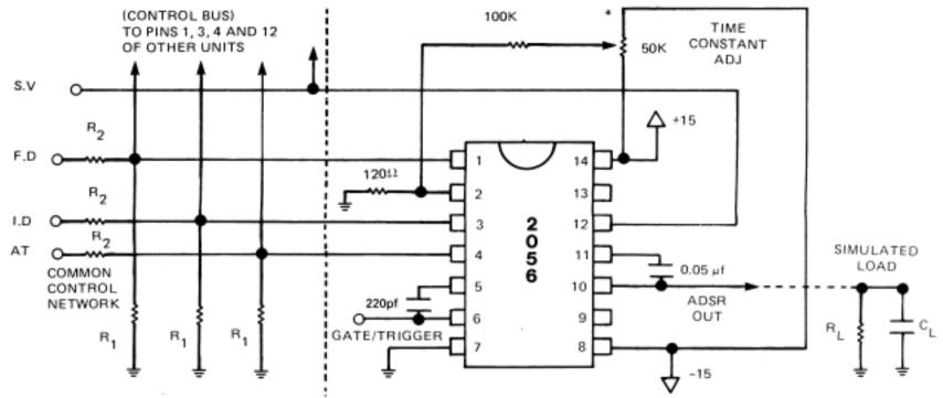
\*Optional: Adjusts for capacitor value and slight unit to unit variation. Ground Pin 2 if not required.
